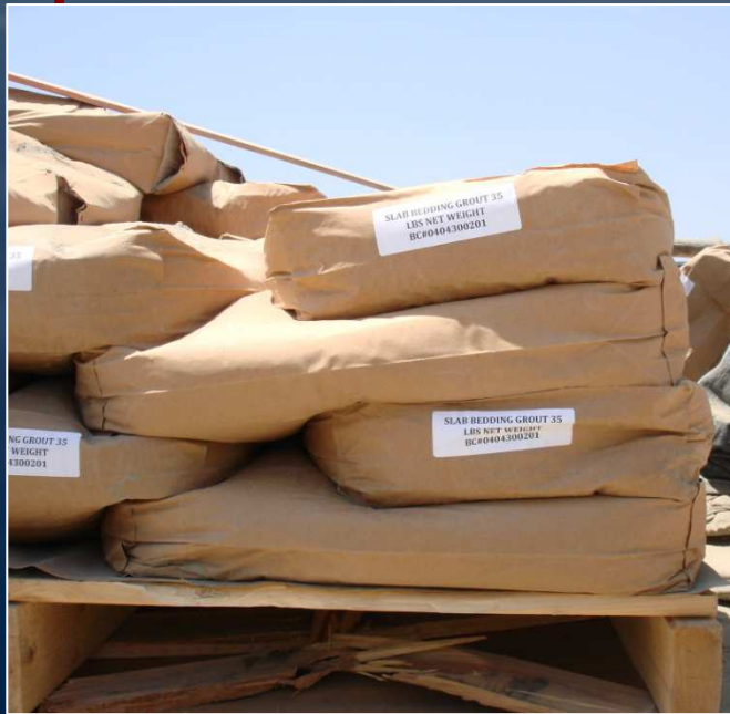
Pre-bagged Bedding Grout (Recommended)
